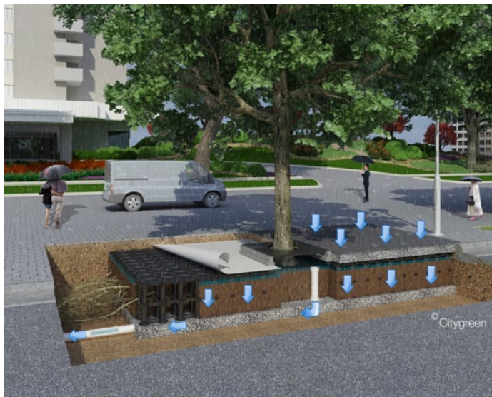
Figure 2: Strata vaults are one option to support healthy trees. (Source: Citygreen)
